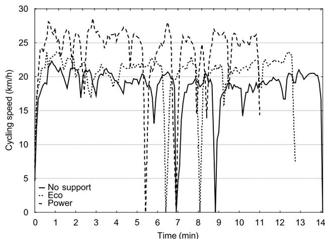
**FIGURE 2**—Typical example of the cycling speed during the cycling test without support, in the eco, and in the power mode.
